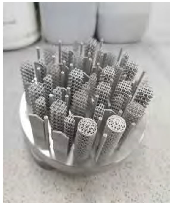
Fig. 1 shows additively manufactured Inconel 718 samples
